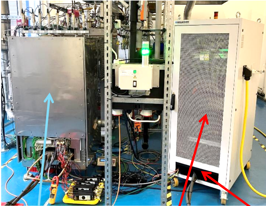
SolydEra LSM Stack Module G8x10 100 Layers - 320 cm 2 10 kWe / 30 kWe Fuel Cell / Electrolysis
