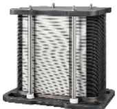
SolydEra LSM Stack Module G8x10 100 Layers - 320 cm 2 10 kWe / 30 kWe Fuel Cell / Electrolysis
